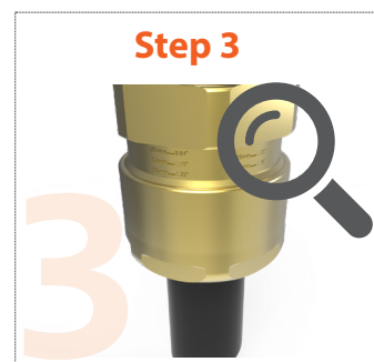
Step 3 The backnut should be level with the marking guide corresponding to its diameter – this can be visually inspected and adjusted as necessary
