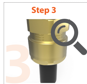
The backnut should be level with the marking guide corresponding to its diameter – this can be visually inspected and adjusted as necessary
