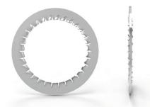
High quality metallic serrated washers designed to designed to protect against loosening of cable gland or locknut in vibrating applications. Often used when mounting a cable gland mounted to a thin wall enclosure, fitted internally with a locknut.
