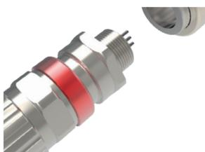
**5 Running Coupler** - Allows the connector to be installed onto a pre-assembled cable gland. Connector is front loaded and includes locking engaging nut.
