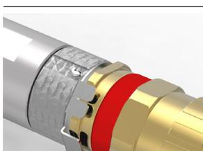
**8 Anti-Rotation Device** - Connector plugs and receptacles come complete with anti-rotation ring, which when fitted between the connector and gland, helps to eliminate the possibility of the gland loosening, locking this in position.
