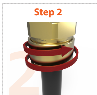
Step 2 Tighten backnut until a seal is formed onto the cable, then tighten one further turn
