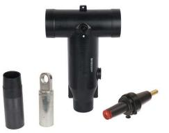
15 kV 600 Amp Load Break Reducing Tap Plug Kit with Test Point. Cable insulation range 0.850 in - 1.050 in. Kit includes Tbody, insulating plug with cap, compression lug, threaded stud, cable adapter, and shield adapter kit
