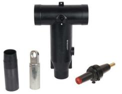
15 kV 600 Amp Load Break Reducing Tap Plug Kit with Test Point. Cable insulation range 1.280 in - 1.430 in. Kit includes Tbody, insulating plug with cap, compression lug, threaded stud, and cable adapter
