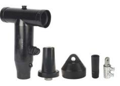
35kV 600A T-Body Kit, with Test Point, Cable Insulation Diameter Range = 1.485 - 1.595 Inches. Kit includes T-body with Testpoint, Cable Adapter, Aluminum Stud, Insulating Plug with Cap, and Shear Bolt connector for 500 Stranded or Compressed and 600 Compact conductor.
