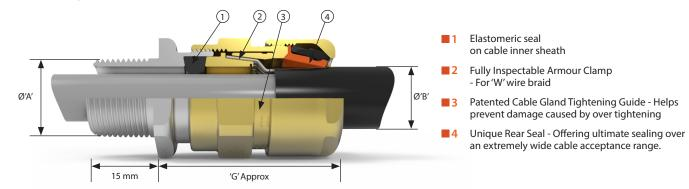
The 153/X Cable Gland is general purpose cable gland for use with wire braid 'X', elastomer and plastic insulated cables. The gland provides an elastomeric seal on the cable inner sheath, and a low smoke, zero halogen IP and retention seal onto the cable outer sheath. See technical section for installation rules and regulations
