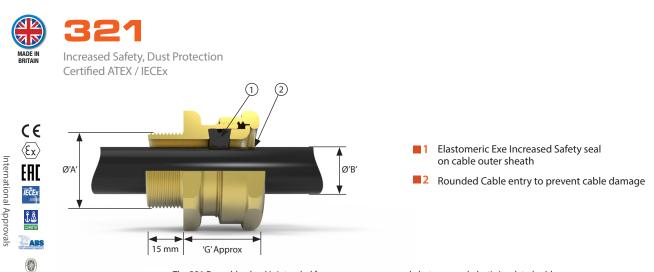
The 321 Exe cable gland is intended for use on non-armoured elastomer and plastic insulated cables. This cable gland may be used with braided cables where the braid and outer sheath pass into the enclosure. The braid must then be suitably terminated inside the enclosure.
