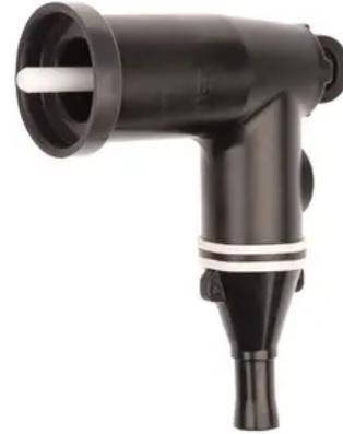
Load Break Elbow, 200 Amp, 15 kV, with Test Point, Long Bimetal Contact, Shield Adapter Kit, Cable Insulation Diameter range = 0.760 - 1.135 inches, 3/0 Solid or Compacted and 2/0 Stranded or Compressed
