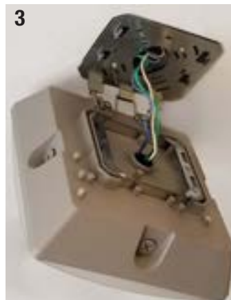
Complete wiring connections.
