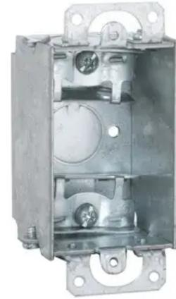
3 in. x 2 in. Switch Box, Gangable, 2 in. Deep, One 1/2 in. KO & AC/MC/Flex Clamps, Plaster Ears
