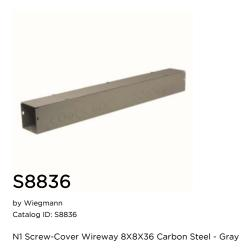
• Bodies and covers are fabricated from 14 gauge steel. S Series screw cover design covers held firmly in place with captivated screw fasteners. Straight sections with knockouts are provided on side walls on wireways.
