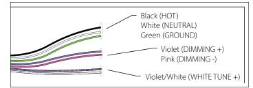
SpectraSync Tunable White luminaires are provided with two 0–10V circuits. The violet and pink circuit is for wiring to any qualified 0–10V controller for dimming. The violet/white and grey/white circuit is for wiring to any qualified 0–10V controller for Tunable White CCT control.
