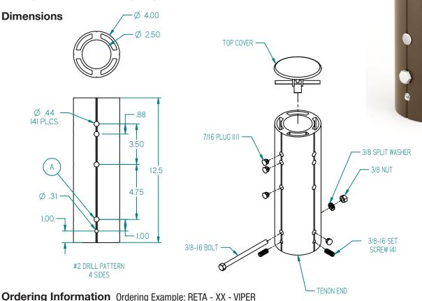
**VIPER** RETA Stocked Fitters RETA-DB-VIPER Series **DRILLING RETA-PS-VIPER ROUND ALUMINUM** BLACK DRILLED QUAD RETA BL TENON TOP FITTER FOR VIPER LED DARK BRONZE DB FOREST GREEN FG GR GREEN PS PLATINUM SILVER RD RED 1 Must provide RAL color number at time of ordering WHITE WH <sup>2</sup> Must provide color chip sample at time of ordering
