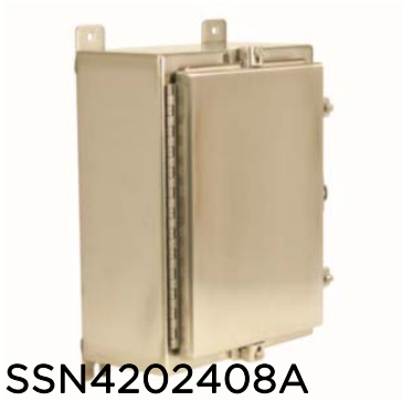
by Wiegmann Catalog ID: SSN4202408A N4X Single Door Wall-Mount Clamp 20X24X8 316 Stainless Steel
