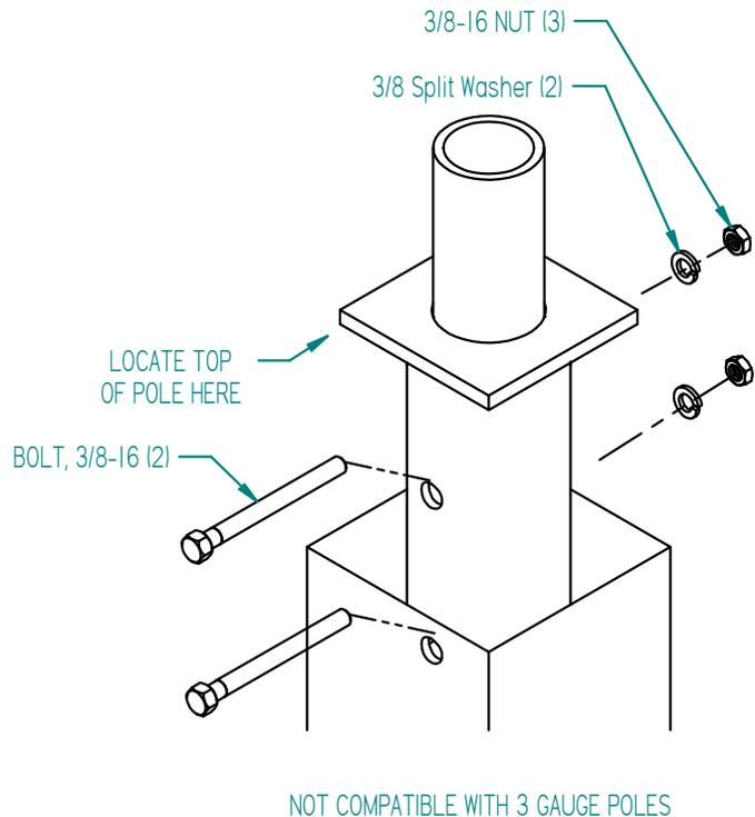
**WARNING:** To avoid damaging supply wiring, drill all necessary holes in poles, arms, or mounting brackets BEFORE pulling supply wires.
