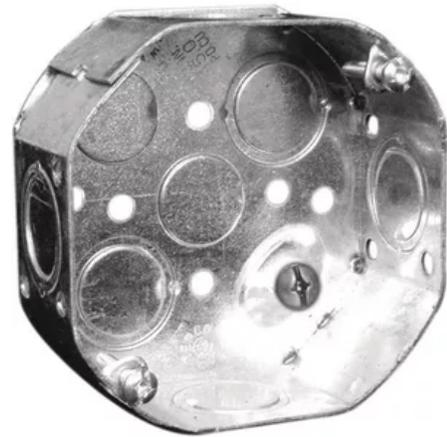
4 In. Octagon Box, 1-1/2 in. Deep, 15 Cu. In., with Raised Ground Screw, with Concentric and 1/2 in. KO (50-Pack)
