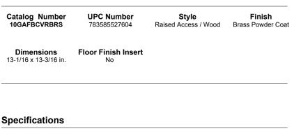
Cover Material Flange height Adjustment Range Load Rating Aluminum 0.25 in. 0 - 1.0 inch 1500 lbs. (w/ 2x safety factor)
