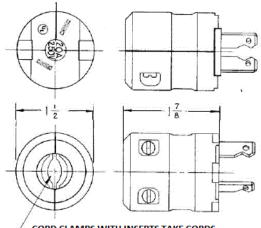
CORD CLAMPS WITH INSERTS TAKE CORDS FROM 19/64 TO 29/64 DIA. & WITHOUT INSERTS FROM 29/64 TO 11/16 DIA.
