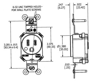
UL Listed to UL498 File No. E2562 Certified to CSA, C22.2, No. 42 File 661 Fed. Spec. W-C-972 NEMA® WD-6 Compliant
