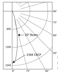
Voltage: 120 Watts: 6.84 Amps: 0.83 Lumens: 470 CBCP: 2344 Beam: 20°
