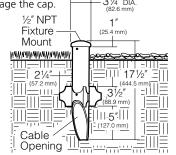
• Low Voltage Spear Mount: Die-cast low copper aluminum with K" NPSM fixture mount. Stainless steel set screw locks fixture into mount. Cable slot allows easy fixture mounting before or after installation in ground. Super TGIC powder coat paint over clear anodizing and titanated zirconium conversion coating.
