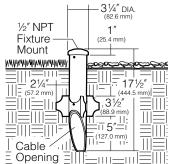
• Low Voltage Spear Mount: Die-cast low copper aluminum with K" NPSM fixture mount. Stainless steel set screw locks fixture into mount. Cable slot allows easy fixture mounting before or after installation in ground. Super TGIC powder coat paint over clear anodizing and titanated zirconium conversion coating.
