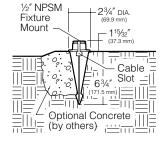
• Low Voltage Surface Mount: Die-cast low copper aluminum with 1/2" NPSM fixture mount. Stainless steel set screw locks fixture into mount. Two holes provided for flat head wood screws. Super TGIC powder coat paint over clear anodizing and titanated zirconium conversion coating.
