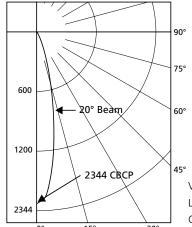
Voltage: 12 Watts: 6.84 Amps: 0.83 Lumens: 470 CBCP: 2344 Beam: 20° CCT: 3000K Efficacy: 69 Lm/W
