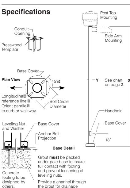
**Pole Construction:** One-piece non-tapered round shaft of low carbon steel (ASTM-A500 Grade B, 42,000 PSI min. yield) with one flush-welded vertical seam. Shaft is welded to a flat steel anchor base (ASTM-36, 36,000 PSI min. yield).
