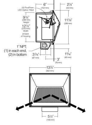
Arrows indicate main thrust of light distribution, in elevation.
