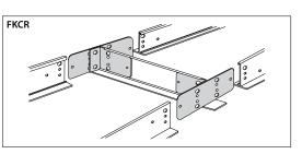
For flanged fixtures in row configurations, the FKCR adapter bracket kit is required in addition to the FK24 kit. Order one less FKCR than the total number of fixtures in row. (Example: Row of two, order (2) FK24 & (1) FKCR)
