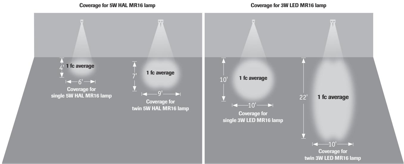
Meets Life Safety Code minimum illuminance of 0.1 fc and average illuminance of 1.0 fc. Assumes open space with no obstructions, mounting height of 7.5', ceiling height of 9' and reflectances of 80/50/20. Photometry files available on the Dual-Lite web site ([www.dual-lite.com](http://www.dual-lite.com)).
