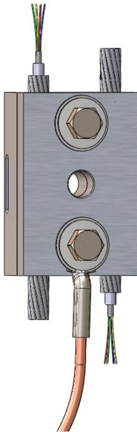
The **CPI OPGW Grounding Down Lead Clamp** is designed to connect OPGW to the pole or structure as it is routed down to the splice-box. The grounding lug can be attached to either bolt point and adds an additional layer of safety by grounding out any voltage that may be picked up through the OPGW as it travels through the phases.
