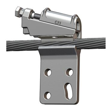
**CPI Aluminum Pad Tap Connectors** are designed to connector Aluminum or Copper conductor to a variety of 2-Hole or 4-Hole NEMA standard devices. Some examples are in mounting sectionalizing switches, connecting compression lugs for risers or various uses in Sub Stations.
