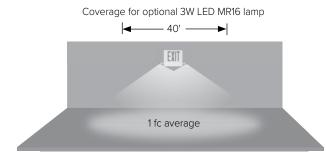
Meets Life Safety Code minimum illuminance of 0.1 fc and average illuminance of 1.0 fc. Assumes open space with no obstructions, mounting height of 7.5', ceiling height of 9' and reflectances of 80/50/20. Photometry files available on the Dual-Lite web site (www.dual-lite.com).
