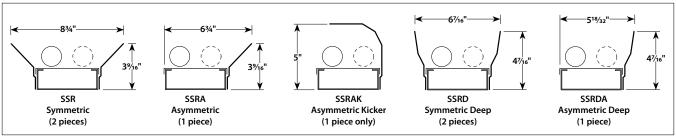
ORDERING GUIDE: Show reflector as option on strip catalog number to provide mounting holes in fixture body. Order reflectors as separate line items.
