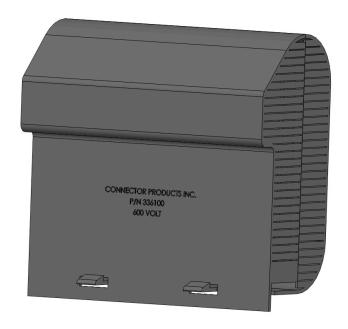
**CPI Tap Covers** are used to electrically insulated Wedge Tap connectors from neighboring connectors on adjacent phases, exposed ground conductors, nearby grounded structures or vegetation. These covers are intended for casual contact only and are not for use as personal protection. Typical applications are 600-volt maximum insulated-conductor overhead applications.
