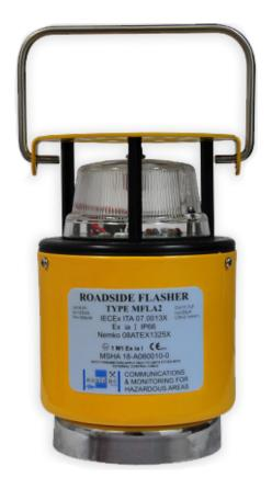
The roadside flasher type MFLA2 is a portable explosion protected Ex ia LED based self-flashing lantern designed for general hazard identification in underground coalmines.
