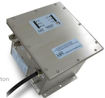
The Austdac Uninterruptible Power Supply (UPS) type 12/NMH/288 has been designed to provide battery backup for equipment located in hazardous areas that operates from a nominal 12Vdc supply. The UPS can support loads up to a maximum of 2.5A.
