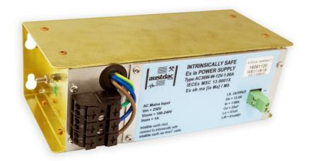
The Power Supply Type AC36W is an intrinsically safe power supply that has a nominal output voltage of 12 volts DC and an output current of up to 3.3A or 16V DC and an output current of up to 1A. The AC36W is an active power supply. The AC36W is suitable for use in Group I and IIB applications. The AC36W power supply may be used to power intrinsically safe apparatus located in zone 0, 1 or 2.
