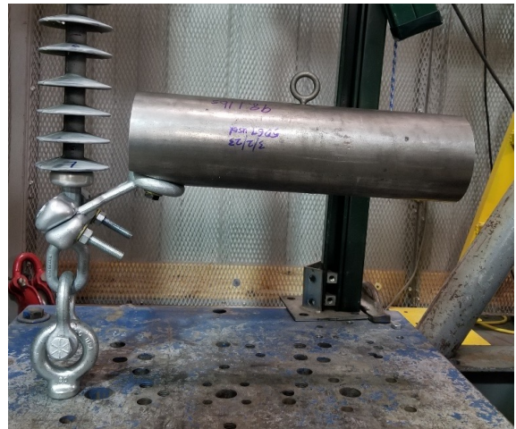
Figure 8: EGLA support hardware under mechanical testing
