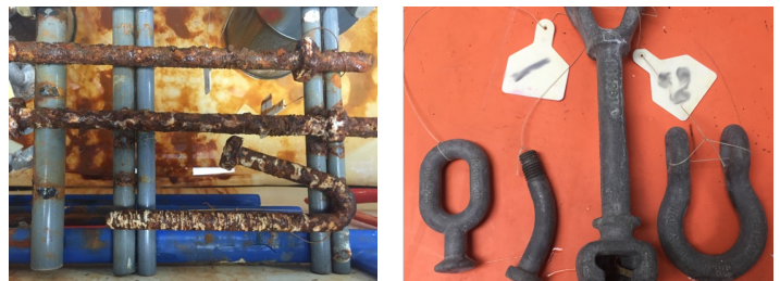
Figure 9: HDG test samples (left), TDG samples (right) after 2850 hours salt fog
