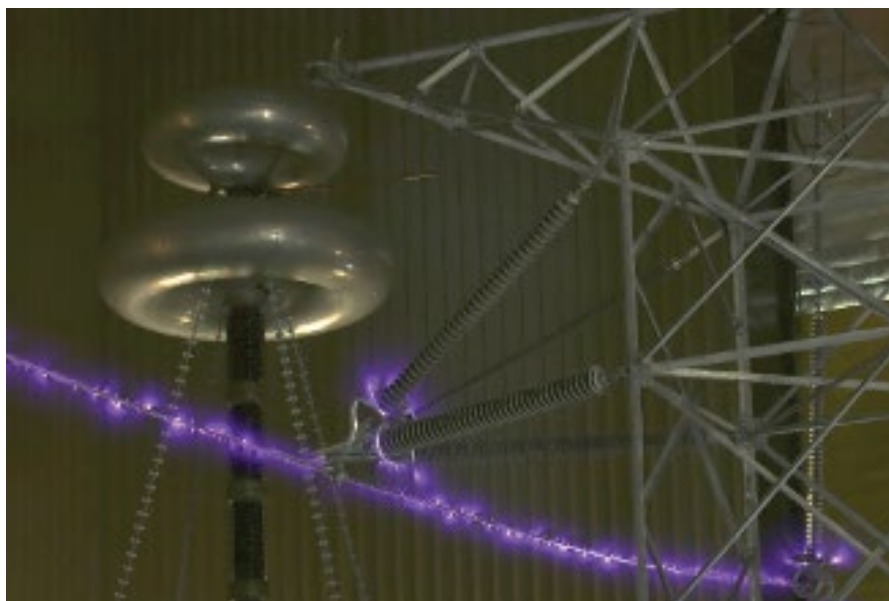
Figure 08 – Generalized corona effect forced by much higher voltage – Only the most extreme parts on the insulator rings and the external point on the nose protection ring shows ionized activity in this extreme condition above voltage class level.
