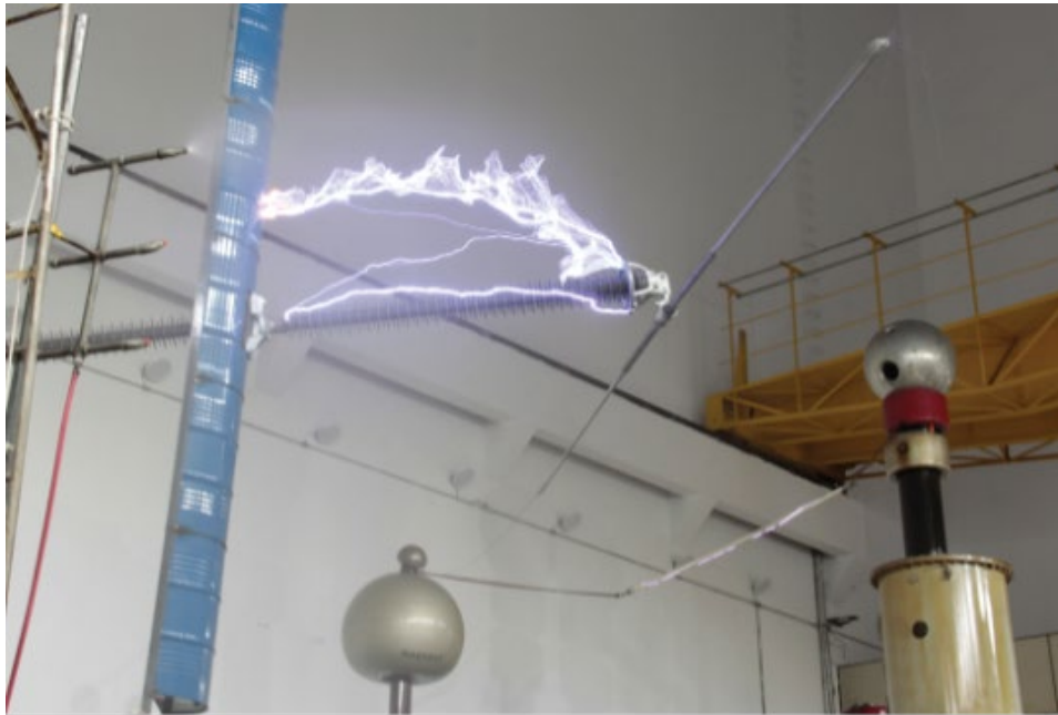
Figure 12 - Wet power frequency flashover voltage on a 230 kV 12° angle upside tilted line-post insulator - The arc voltage path is different than a suspension chain
