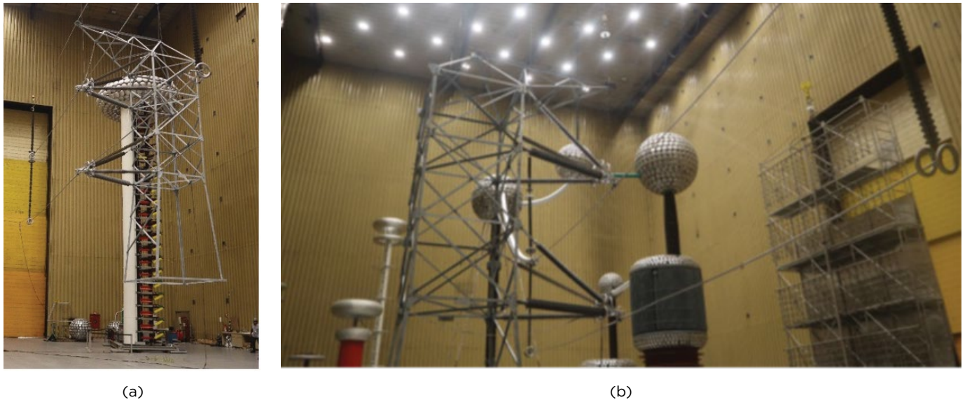
Figure O6 - Tower mounted at HV LAB for impulse (a) and power frequency (b) voltage tests [14]
