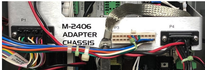
Figure 19 M-2406 Adapter Chassis P1, P3, and P4 Connections
