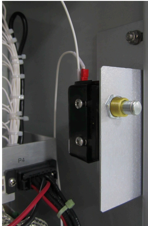
Figure 36 Back Door Switch 2 Mounted on Bracket
