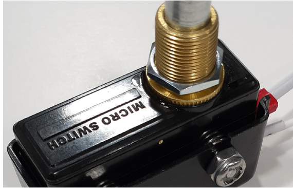
Figure 33 Switch Mounting Nut #1 Installed
