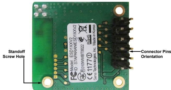
Figure 8-3 Bottom of Bluetooth Serial Module, Connector Orientation
