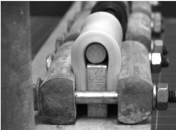
[ Figure 2 ] Silicone rubber corona cutting sample mounted, prior to placement of electrode.
