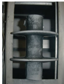
Chalking on polymer housing after QUV testing
