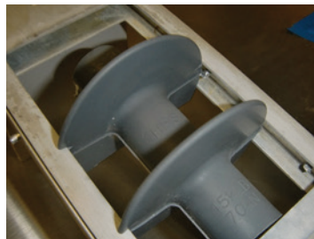
Insulator sample before testing in the QUV chamber
