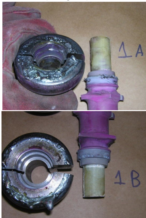
Figure 5: Power Arc Test Results of Quadri*Sil Insulator Sealing System
