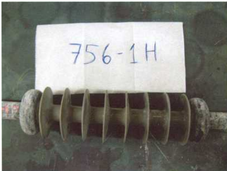
Figure 3A: Photograph of Housing: Tracking and Erosion Test Horizontal Insulator (after test)
