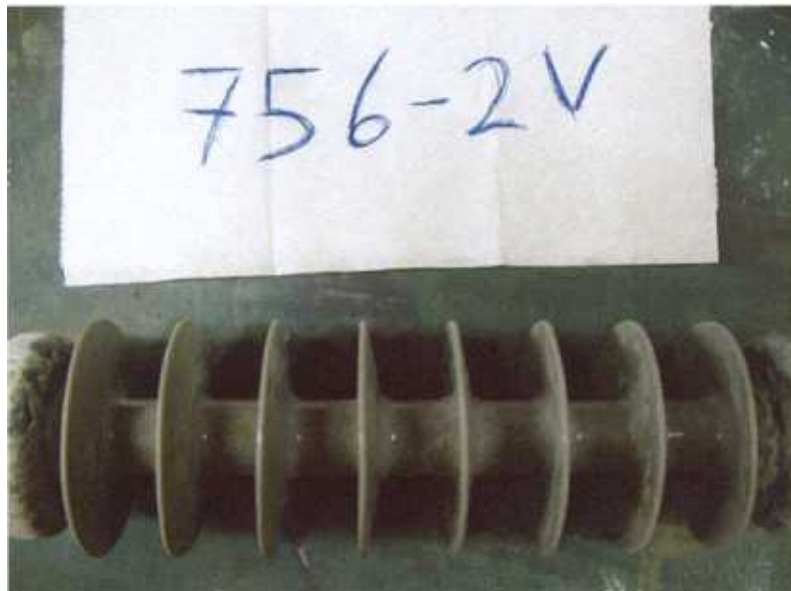
Figure 3B: Photograph of Housing: Tracking and Erosion Test Vertical Insulator (after test)
