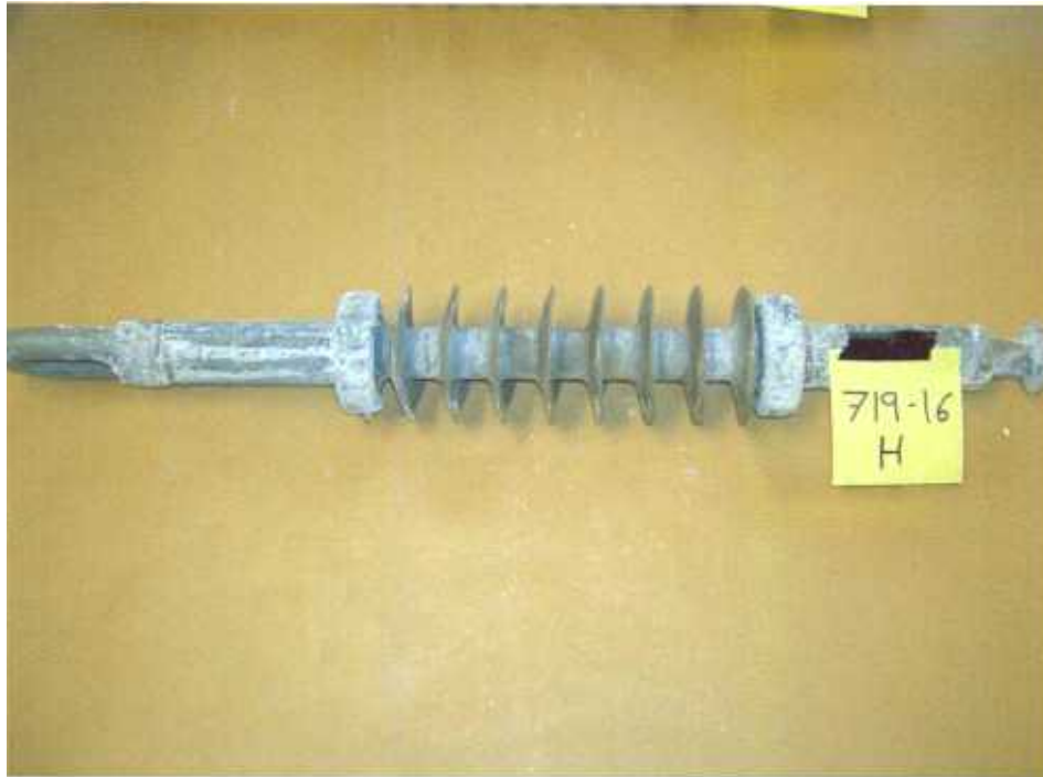
Figure 3b: Photograph of Housing: Tracking and Erosion Test Insulator (passed)
