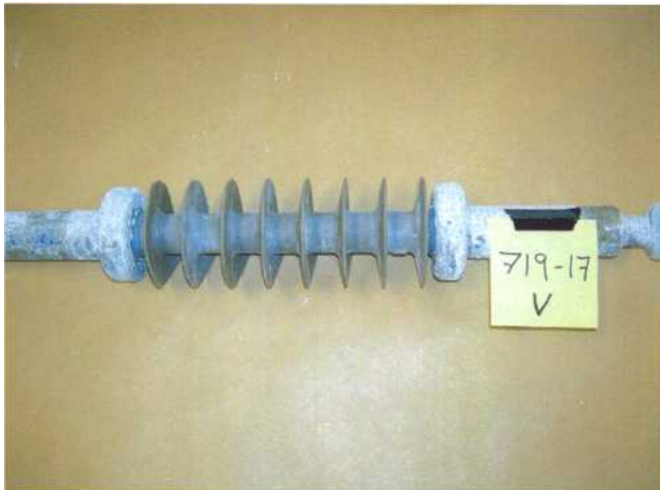
Figure 3c: Photograph of Housing: Tracking and Erosion Test Insulator (passed)
