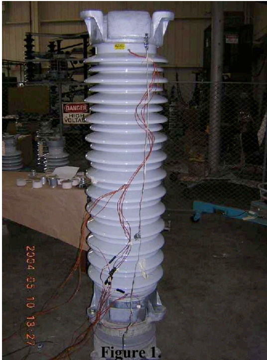
Figure 1. Fully assembled unit with thermocouples between resistors at 3 locations
