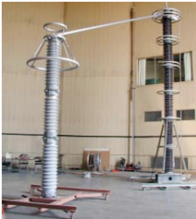
Figure 1. 420 kV rated arrester (RIV coupling capacitor in rear)
