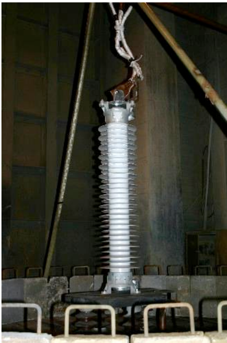
Figure 2. Test sample mounted in test chamber
