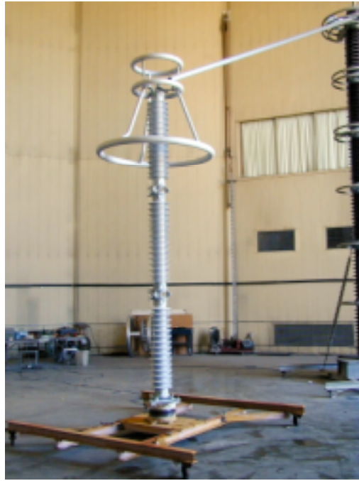
Figure 1. 312 kV rated arrester
