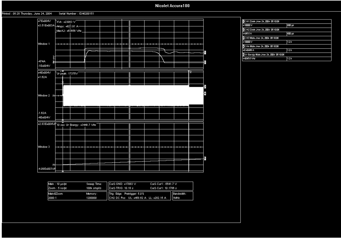
Figure 4. Oscilloscope of second line discharge and application of U_r for section 1
