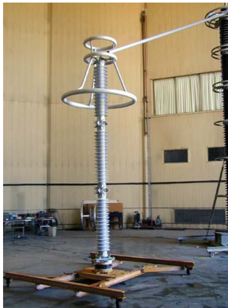
Figure 1. Arrester installed for RIV test
