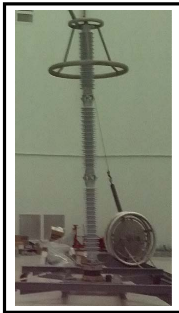
Figure 1. Arrester installed for RIV test
